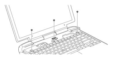
Figure 8-8 Removing the keyboard (1)
